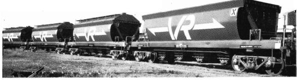
Fifty-five multi-purpose hopper wagons are being built at Newport Workshops. The wagons, designed by Victorian Railways' Rolling Stock Engineer's section, are for four types of traffic, but the specialised equipment for each type is readily interchangeable.
