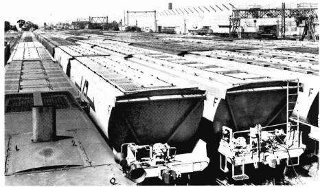
TOGETHERNESS IN TESTING. Row upon row of GJF hopper wagons have their brakes hydraulically tested at North Williamstown. Below is the panel of pressure gauges which indicate whether all brakes are in working order.
