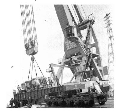
An 80-tonne transformer is unloaded on to a special QS wagon at Appleton Dock, before being railed to Redcliffs.
